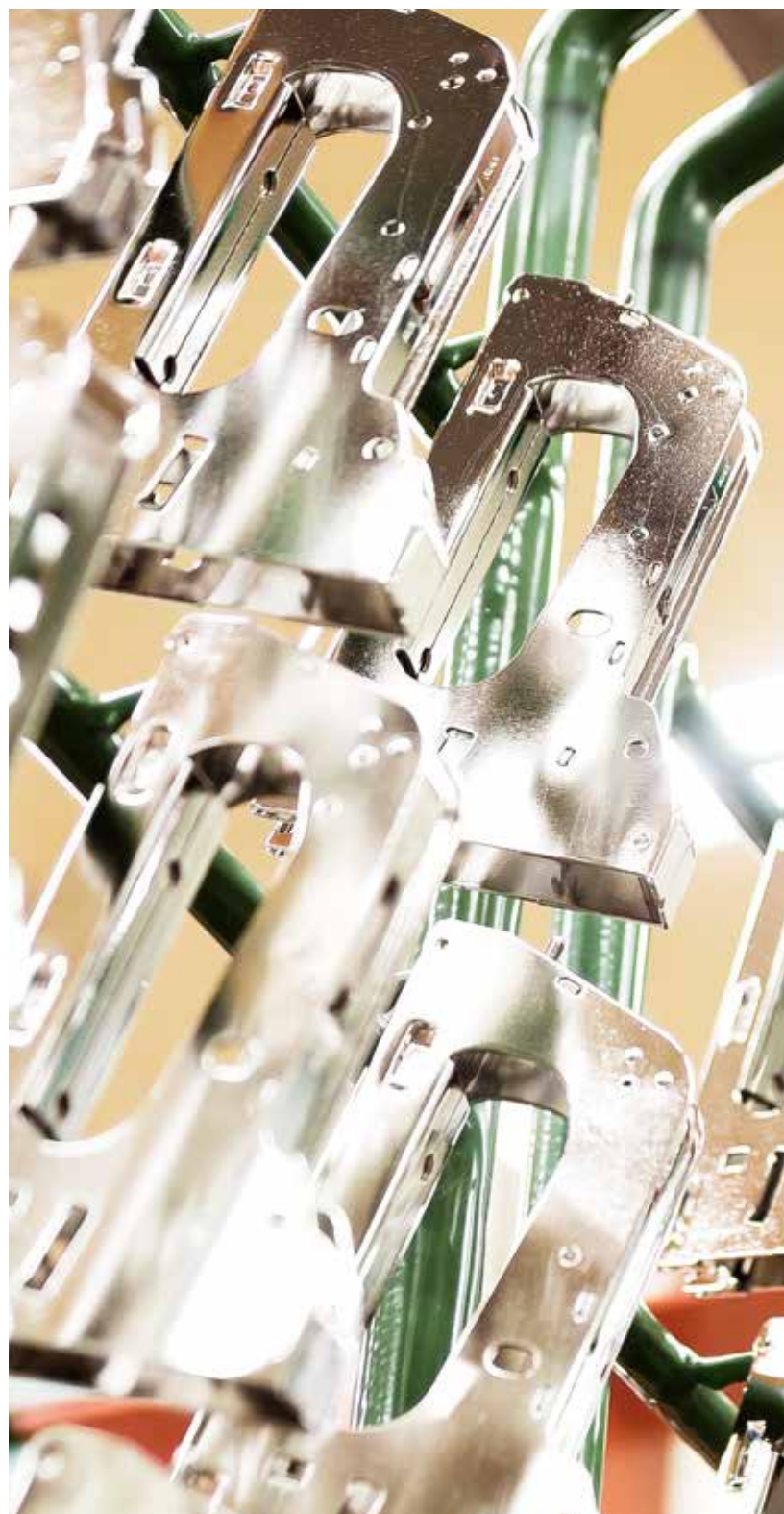
Product-adapted suspension system for an optimal surface finish at a trivalent chromium plating plant.
